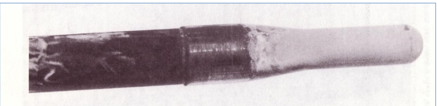
Thermowell of a “worst case” platinum resistance thermometer removed from the reactor coolant system hot-leg showed radioactive surface deposits (right). This device was exposed to superheated steam during the accident; however, its calibration or its time response was not adversely affected by the accident.
